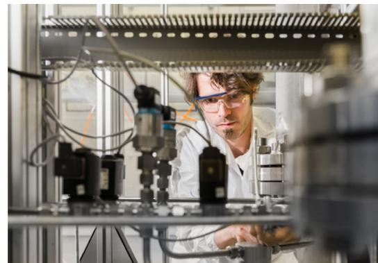
*Assembly of Pressure Swing Adsorption System (rights by Photograph: [www.eventfotograf.in](http://www.eventfotograf.in) / ©JRF e.V.)*
